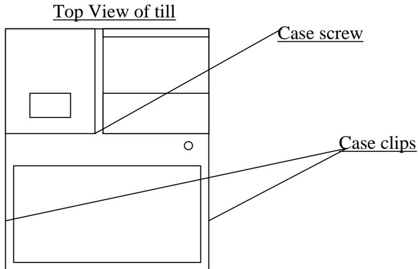
Release the case clips by pressing upwards where indicated on the drawing above.
